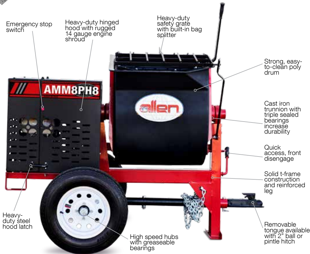
Our spiral mixer design offers a faster more consistent mix.
