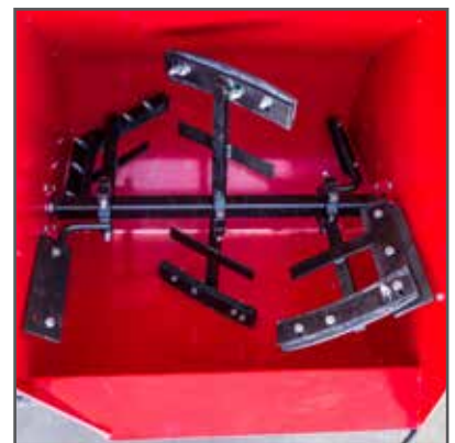
Our standard paddle design includes extra paddles on each end for a better mix.
